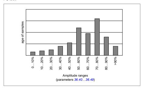
Amplitude logger 1 is fixed to monitor motor current, and cannot be reset. With amplitude logger 1, 100% corresponds to the maximum output current of the drive  $(I_{\text{max}})$ , which is listed in the *Hardware manual* of the drive. The measured current is logged continuously. The distribution of samples is shown by parameters 36.20...36.29.
