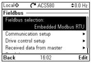
Use the settings in the **Fieldbus** submenu to use the drive with a fieldbus:
