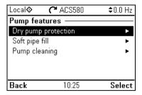
Use the **Pump features** submenu to adjust pump-related settings, such as pump protection functionalities, soft pipe fill or pump cleaning configurations.
