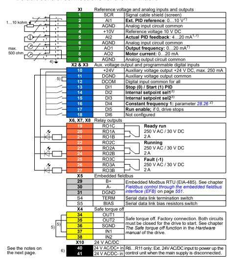
R1...R5: 0.2...2.5 mm<sup>2</sup> (terminals +24V, DGND, DCOM, B+. A-) 0.14...1.5 mm<sup>2</sup> (terminals DI. Al. AO. AGND. RO. STO) R6...R11: 0.14...2.5 mm<sup>2</sup> (all terminals)
