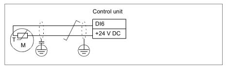
For wiring of the sensor, see the Hardware manual of the drive.
