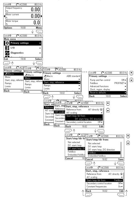
The sections below provide detailed information about the contents of the different submenus available in the Primary settings menu.
