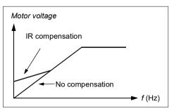
In vector control, no IR compensation is possible or needed as it is applied automatically.
