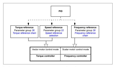
The following is a more detailed representation of the reference types and control chains. The page numbers refer to detailed diagrams in chapter *Control chain diagrams*.
