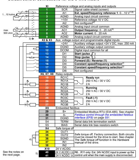
R1...R5: 0.2...2.5 mm<sup>2</sup> (terminals +24V, DGND, DCOM, B+. A-) 0.14...1.5 mm<sup>2</sup> (terminals DI. Al. AO. AGND. RO. STO)
