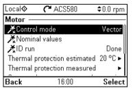
Use the **Motor** submenu to adjust motor-related settings, such as nominal values, control mode or thermal protection.
