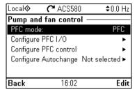
The Pump and fan control submenu contains settings for the Pump and fan control logic. The Pump and fan control is supported in external control location EXT2 only.
