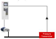
Select the refrigerant gas (81.35), gas pressure source (81.36) and the selected gas pressure unit (81.37). Check the actual gas temperature with parameter 81.30.
