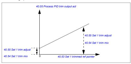
Note: In the above graph, it is assumed that the PID output is limited/stable at 100. This is for understanding purpose only. In real case scenario, PID output can vary based on the setpoint and actual.
