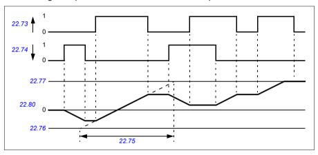
Parameters 22.73 Motor potentiometer up source and 22.74 Motor potentiometer down source control speed or frequency from zero to maximum speed or frequency.
