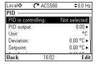
The PID submenu contains settings and actual values for the process PID controller for controlling multiple pumps or fans through the drive's relay outputs.
