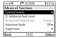
The Advanced functions submenu contains settings for advanced functions, such as triggering or resetting faults via I/O, signal supervision, using the drive with timed functions, or switching between several entire sets of settings.
