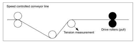
You must link the trimmed output from PID to the speed chain manually if PID trimmed output is used for trimming speed. Set the below parameters as follows:
