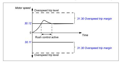
The function is based on a PI controller. The proportional gain and integration time can be defined by parameters. Setting these to zero disables rush control.
