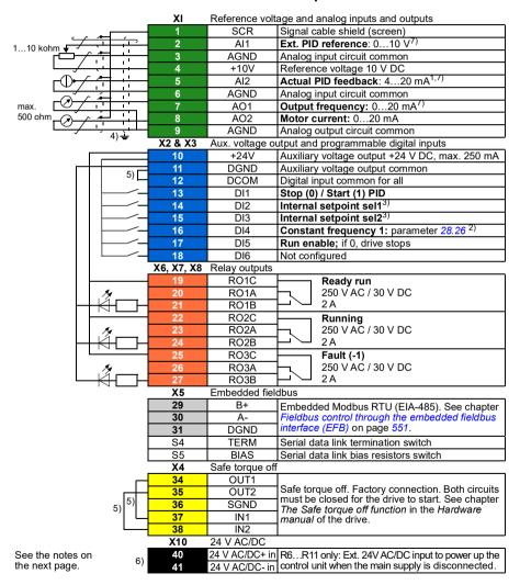
R1...R5: 0.2...2.5 mm<sup>2</sup> (terminals +24V, DGND, DCOM, B+. A-) 0.14...1.5 mm<sup>2</sup> (terminals DI. Al. AO. AGND. RO. STO) R6...R11: 0.14...2.5 mm<sup>2</sup> (all terminals)
