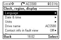
The Clock, region, display submenu contains settings for language, date and time, display (such as brightness) and settings for changing how information is displayed on screen.
