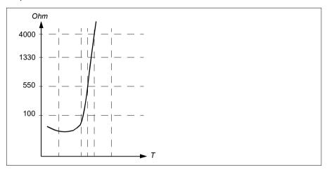
Isolated PTC sensor can also be connected directly to digital input DI6. At the motor end, the cable shield should be earthed through a capacitor. If this is not possible, leave the shield unconnected. See section *Insulation* on page 195.
