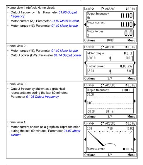
You can replace parameters in the Home view displays with other parameters or create new Home view displays showing selected parameters.
