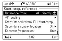
Use the **Start**, **stop**, **reference** submenu to set up start/stop commands, reference. and related features, such as constant speeds or run permissions.
