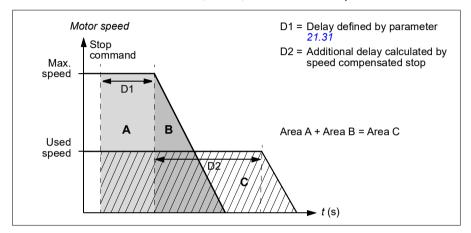
Speed compensation does not take into account shape times (parameters 23.32 Shape time 1 and 23.33 Shape time 2). Positive shape times lengthen the distance traveled.
