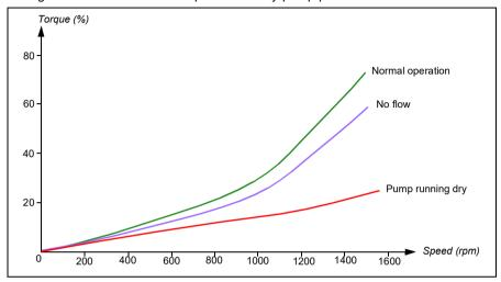
The dry pump can be detected using the underload curve, low level mechanical switch and pressure sensor.
