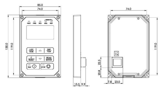
Figure 11.5.3 Dimensions of LCD keypad (IP55)
