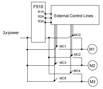
Figure 4.4.118 Cycle modes of inverter pump in the control board
