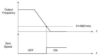
Figure 4.4.23 Zero-speed operation
