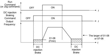
Figure 4.4.21 DC braking timing diagram
