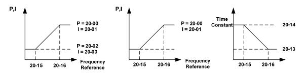
Figure 4.4.96 ASR gain setting (SLV mode)
