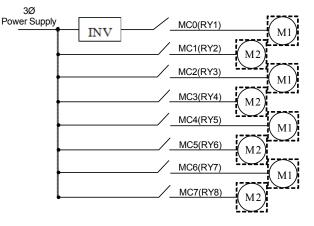
Figure 4.4.116 Fixed modes of inverter pump
