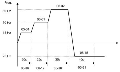
Figure 4.4.44 Single cycle automatic operation (continuous)
