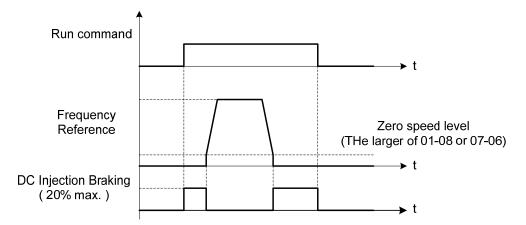
Figure 4.4.84 Zero-speed braking operation
