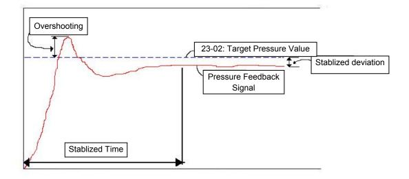
Figure 4.4.103 Diagram of pressure feedback value
