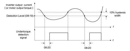
Figure 4.4.64 Low torque detection operation
