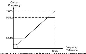
Figure 4.4.5 Frequency reference upper and lower limits
