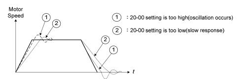
Figure 4.4.97 System response of ASR proportion gain
