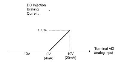
Figure 4.4.34 DC braking current adjustment
