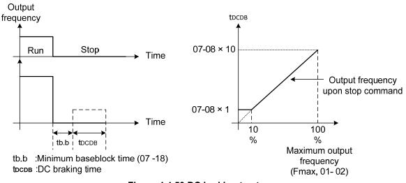
Figure 4.4.50 DC braking to stop
