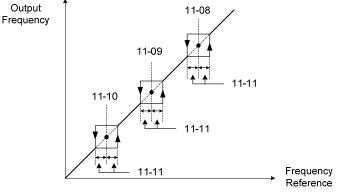
Figure 4.4.77 Jump frequency operation
