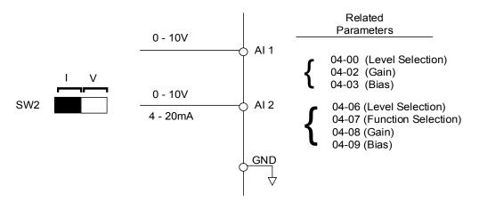
Figure 4.4.25 Analog inputs and related parameters
