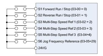
Figure 4.4.14 Control Terminal Wiring Example
