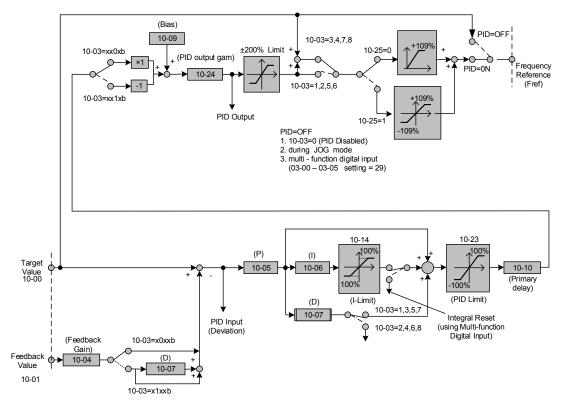
Figure 4.4.72 PID control block diagram
