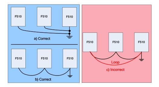
Figure 3.3.7.2 F510 Inverter Grounding
