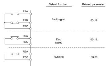
Figure 4.4.22 Multi-function digital output and related parameters
