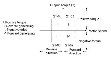
Figure 4.4.101 Torque limit setting
