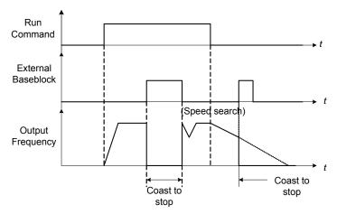
Figure 4.4.19 External base block operation
