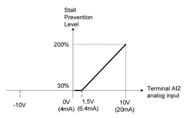
Figure 4.4.36 Stall prevention level adjustment during operation
