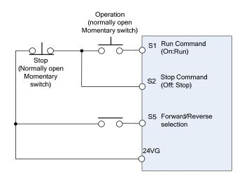
Figure 4.4.2 Wiring example of 3-wire
