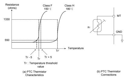
Figure 4.4.66 Protection of motor overheating
