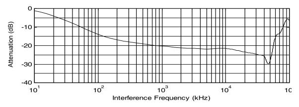
Figure 11.3.1 Frequency attenuation characteristics (10 windings case)
