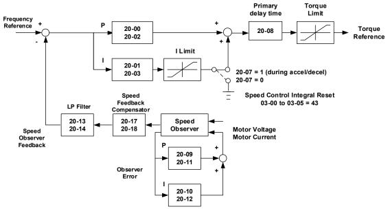
Figure 4.4.95 ASR block diagram (SLV mode)
