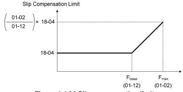
Figure 4.4.91 Slip compensation limit
