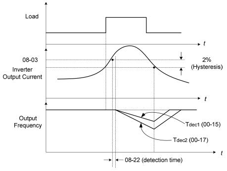
Figure 4.4.60 Stall prevention selection in operation
