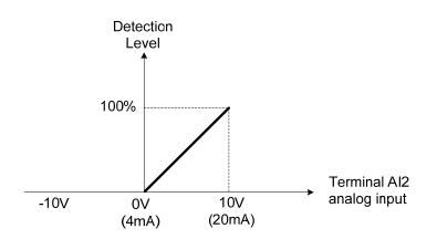
Figure 4.4.35 Over-torque/less torque detection level adjustment
