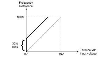
Figure 4.4.31 Frequency Reference bias adjustment (example)
