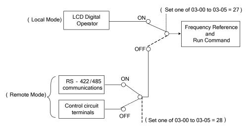
Figure 4.4.20 Remote mode operation selection
