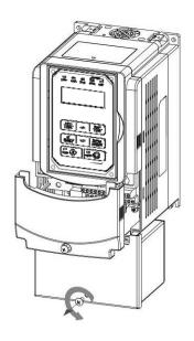
Step 3: Unscrew filter section
