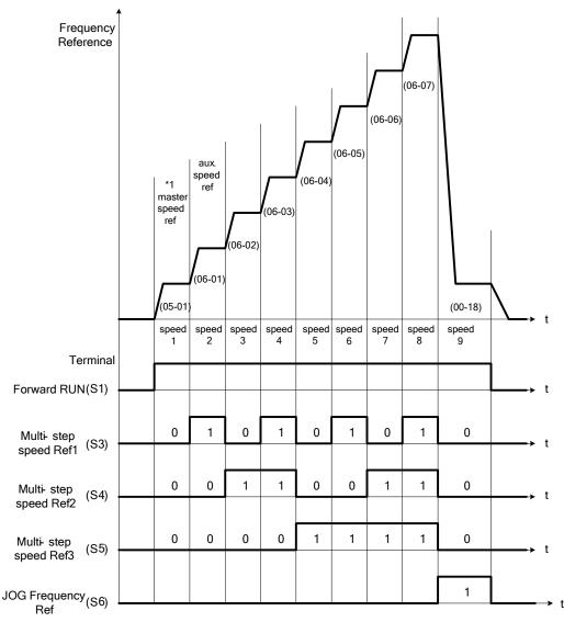
Figure 4.4.15 9-speed timing diagram
