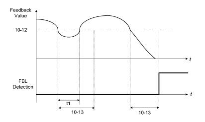
Figure 4.4.73 PID feedback loss detection
