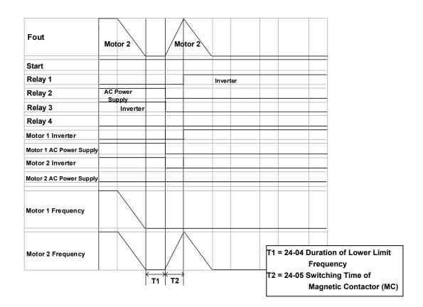
Figure 4.4.123 Diagram of decreasing pump in the fixed modes of inverter pump 4-247
