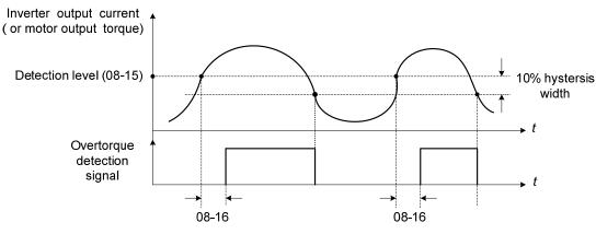
Figure 4.4.63 Over-torque detection operation
