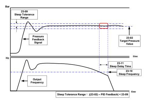
Figure 4.4.105 Diagram for stop time of constant pressure
