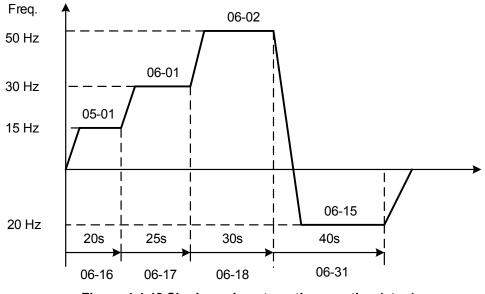
Figure 4.4.42 Single cycle automatic operation (stop)
