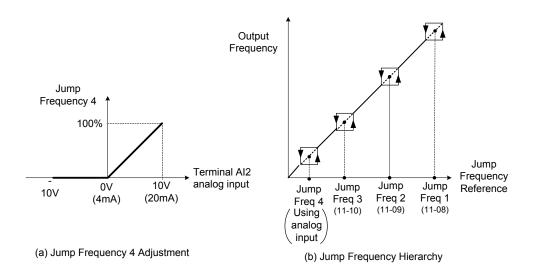
Figure 4.4.38 Jump frequency 4 setting operation
