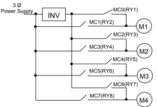
Figure 4.4.117 Cycle modes of inverter pump
