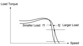
Figure 4.4.90 Slip compensation output frequency
