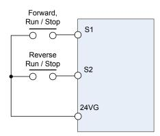
Figure 4.4.1 Wiring example of 2-wire
