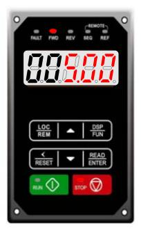
Fig 5.1: LED Keypad (Stopped)
