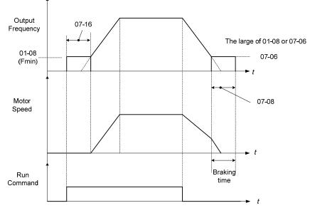
Figure 4.4.47 DC braking operation
