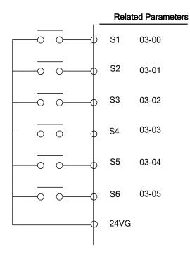
Figure 4.4.13 Multi-function digital input and related parameters
