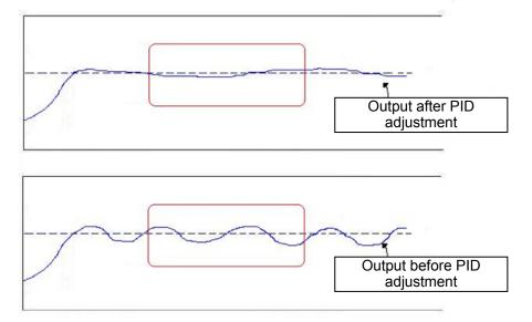
Figure 4.4.104 Diagram for PID parameter adjustment
