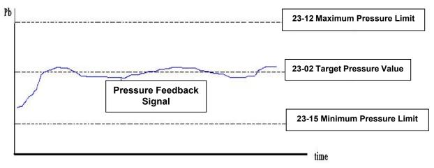
Figure 4.4.106 Diagram for pressure feedback limit
