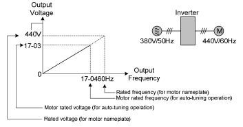
Figure 4.4.89 Rated voltage and frequency settings
