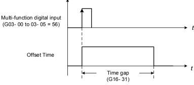
Figure 4.4.88 Operation of offset time
