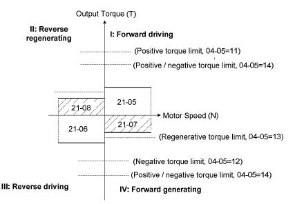
Figure 4.4.102 Analog input torque limit (Al2)
