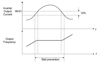
Figure 4.4.57 Stall prevention during acceleration
