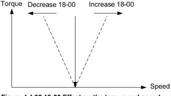
Figure 4.4.92 18-00 Effect on the torque and speed
