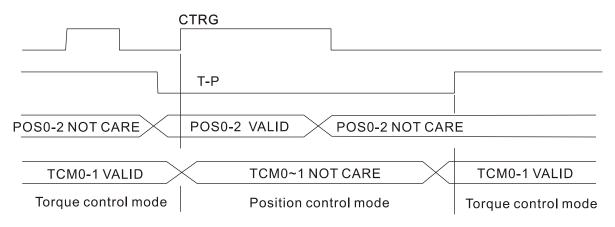
Figure 3.: Torque / Position Control Mode Selection
