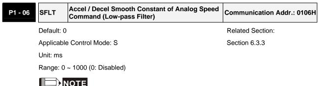
If the setting value of parameter P1-06 is set to 0, it indicates the function of this parameter is disabled and the command is just By-Pass.
