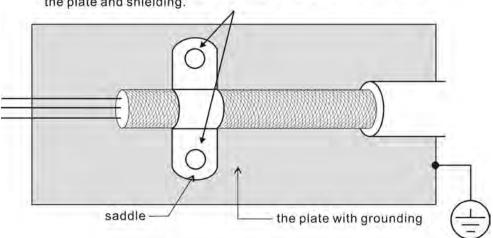
Remove any paint on metal saddle for good ground contact with the plate and shielding.
