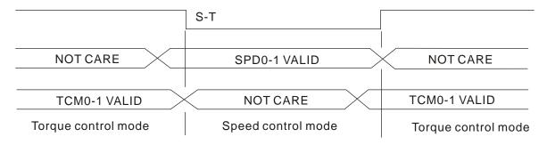
Figure 2. : Speed / Torque Control Mode Selection
