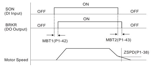
Timing chart for using servo motor with electromagnetic brake:
