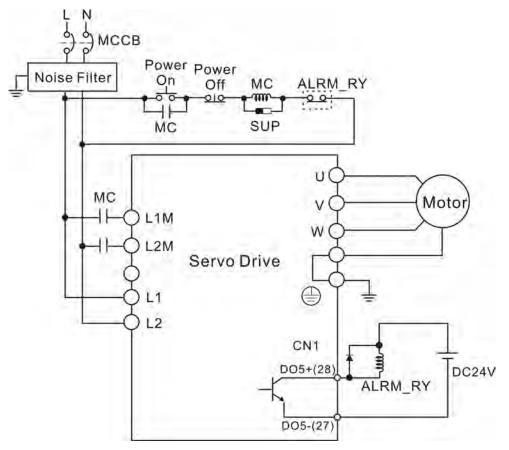
Figure 3.5 Three-Phase Power Supply (all 220V models)
