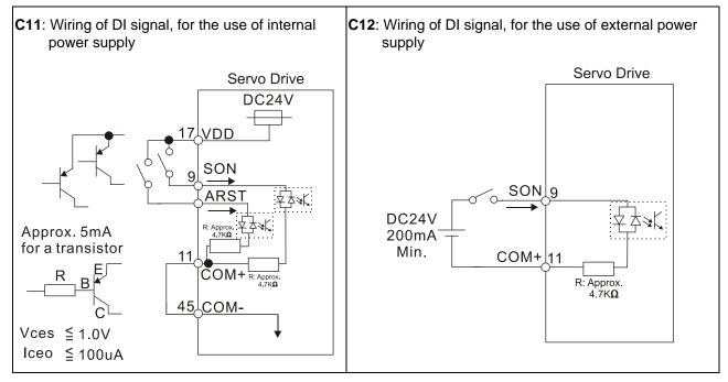
> Caution: Do not use dual power supply. Failure to observe this caution may result in damage to the servo drive and servo motor.
