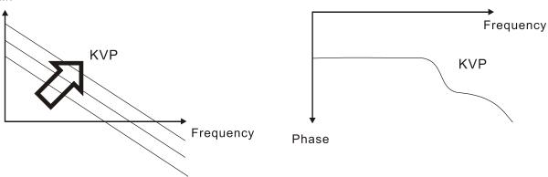
STEP 2 : Fix the value of KVP and adjust the value of KVI.
