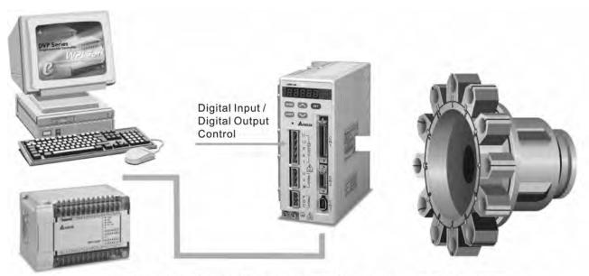
Use communication control (upon software) / Monitor the status of the servo drive
