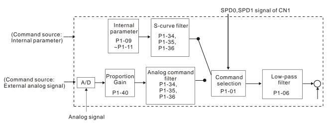
The command source is selected according to the state of SPD0, SPD1 and parameter P1-01 (S or Sz). Whenever the command signal needs to be more smoothly, we recommend the users to use S-curve and low-pass filter.
