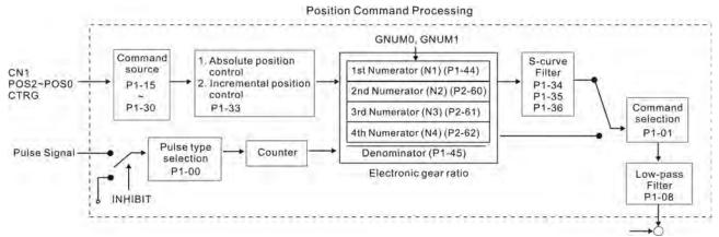
Using parameter can select Pr mode and Pt mode. Electronic gear ratio can be set in both two modes to set proper position revolution. ASDA-AB series servo drive also provides P-curve and low-pass filter, which are used whenever the motor and load need to be operated more smoothly. As for the information of electronic gear ratio, P-curve and low-pass filter, please refer to the following sections 6.2.4, 6.2.5 and 6.2.6.
