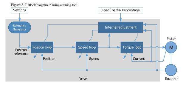
The reference generator plans an appropriate position reference according to the settings of relevant parameter.
