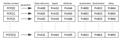
The pulse reference defines the number of pulses of the contact, the speed defines the running speed of the contact, the attributes defines the motion attribute of contact, the acceleration and jerk define the acceleration/deceleration of the contact, and the delay defines the delay time after the contact reference is sent.
