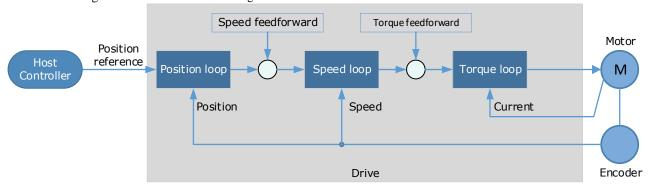
In general, the differential of the position reference is used as the feedforward, you can also set the feed forward by the controller or other application functions.
