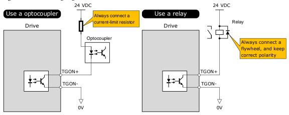
The maximum permissible voltage and current of the ptocoupler output circuit inside the servo drive are as follows:
