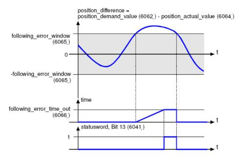
The deviation of the actual position value (position\_actual\_value) from the desired position value (position\_demand\_value) is named following error. As shown in figure above, if for a certain period of time this following error is bigger than specified in the following error window (following\_error\_window) bit 13 (following\_error) of the object statusword will be set to 1.
