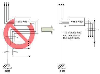
• Connect the Noise Filter ground wire directly to the grounding plate. Do not connect the Noise Filter ground wire to other ground wires.
