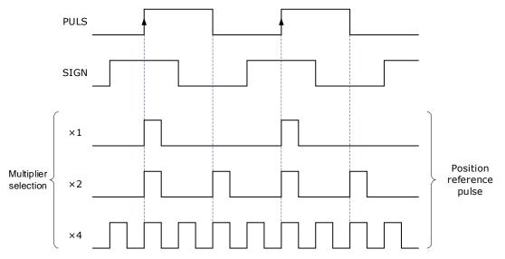
Also, the user can choose whether to invert the PULS signal and SIGN signal using Pn004.3.
