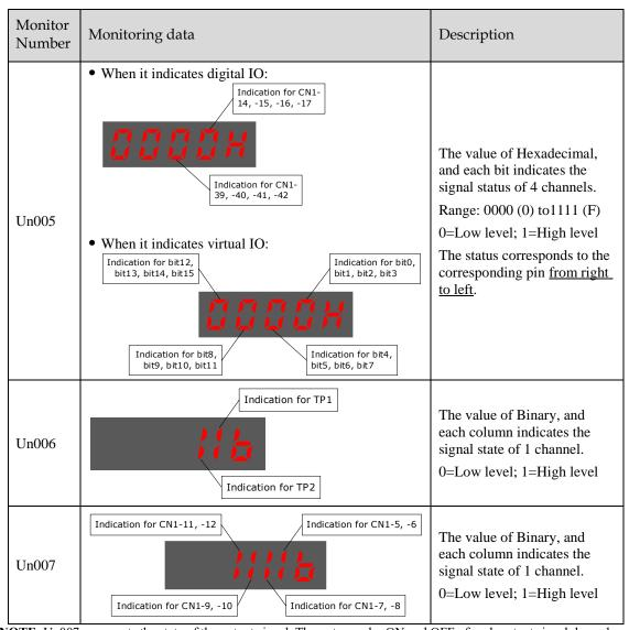
**NOTE**: Un007 represents the state of the output signal. The optocoupler ON and OFF of each output signal depends on whether the output signal is inverted:
