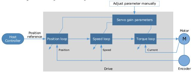
It is necessary to adjust the three-loop control parameters of the Servo from the inside out, that is, the adjustment sequence is  $\boxed{\text{Torque loop}} \rightarrow \boxed{\text{Speed loop}} \rightarrow \boxed{\text{Position loop}}$ . In addition, in order to meet the stability, the bandwidth setting should be the largest in the torque loop, the speed loop is the second, and the position loop is the smallest.
