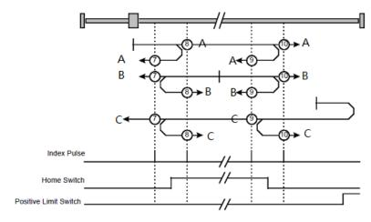
• When the negative limit switch (NOT) is used for homing, the method 11~14 is almost same as method 7~10, and the drive first moves to the negative direction.
