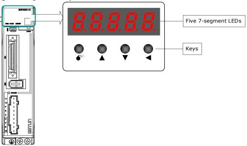
The names and functions of the keys on the Panel Operator are as follows.
