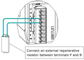
Connect the external regenerative resistor as following to avoid damaging the drive or malfunction.
