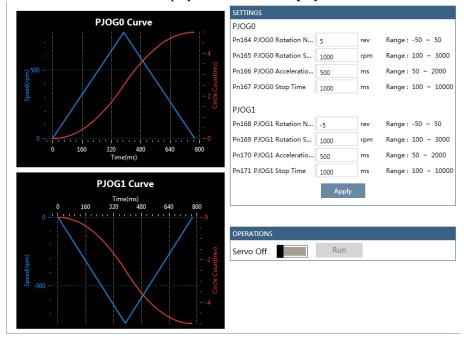
SETTINGS PJOG0 Pn164 PJOG0 Rotation N.. Range: -50 ~ 50 rev Pn165 PJOG0 Rotation S.. 1000 rpm Range: 100 ~ 3000 Pn166 PJOG0 Acceleratio. 500 ms Range: 50 ~ 2000 Pn167 PJOG0 Stop Time Range: 100 ~ 10000 1000 ms PJOG1 Pn168 PJOG1 Rotation N. Range: -50 ~ 50 -5 rev Pn169 PJOG1 Rotation S. . rpm Range: 100 ~ 3000 1000 Pn170 PJOG1 Acceleratio .. Range: 50 ~ 2000 500 ms Pn171 PJOG1 Stop Time Range: 100 ~ 10000 1000 ms
