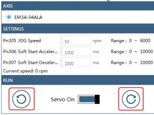
Click and hold the button or can run the Motor continuously, and the Motor can stop running when you release the button.
