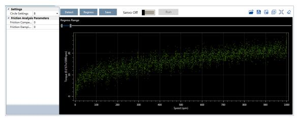
Step 9 Move Regress Range for setting a proper analysis range of Speed.
