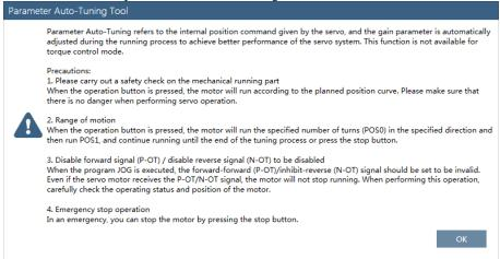
Step 3 The Auto-Tuning Tool window will be displayed in Function Display Area.
