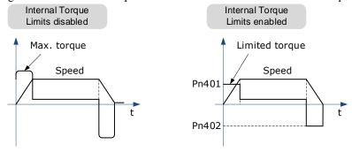
[Note] If the setting of Pn401 or Pn402 is too low, the torque may be insufficient for acceleration or deceleration of the Motor.
