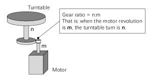
Because the turntable moves in only one direction, the upper limit to the number of revolutions that can be counted by an absolute encoder will eventually be exceeded.
