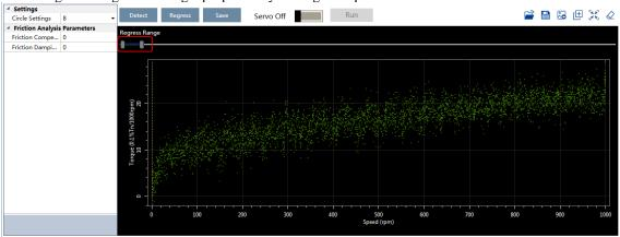
Step 10 Click Regress for calculating the Friction Compensation Gain and Friction Damping Proportion.
