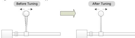
This function is based on the Model Following Control. According to the relationship between the load position and the Motor position in the Model Following Control, aiming at controlling the stability of the load position, and correcting the position reference, as well as the feedforward generated by the Model Following Control. Figure 8-22 shows the block diagram of using the Load Oscillation Suppression.
