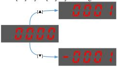
NOTE: the offset can be adjusted from -1024 to 1024.
