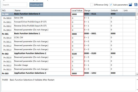
Step 4 在 Before importing parameters into the Drive, you can edit and download the parameters.
