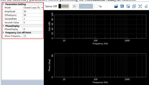
Step 3 Set the necessary parameters before performing the **Mechanical Analysis** function.
