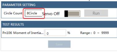
Step 4 Click Servo Off / Servo On for supplying power to the Motor.
