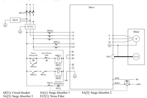
$\begin{array}{lll} KM[1]: \mbox{Magnetic Contactor (for control power supply)} & \mbox{KM[2]: Magnetic Contactor (for main circuit power supply)} \\ Ry[1]: \mbox{Relay} & \mbox{PL[1]: Indicator lamp for display} \end{array}$
