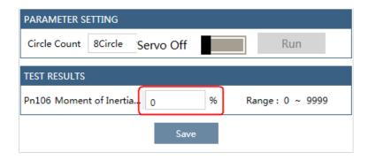
Step 7 Click Save to write the value into the parameter Pn106 of the Drive.
