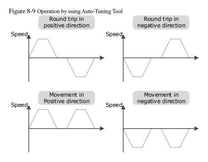
You shall set the Rotations (Pn164 and Pn168) and Max Speed (Pn165 and Pn169) to a proper value. If the Rotations is set too small or the Max Speed is set too large, it is possible that the maximum speed set cannot be reached. In this case, it is necessary to increase the Rotations or decrease the Max Speed.
