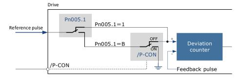
Inhibit (INHIBIT) is switched via/P-CON signal:
