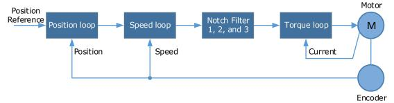
Figure 8-19 shows the relevant parameters for the notch filter. Since the notch filter can attenuate the signal at the notch frequency, if you set a proper frequency (Pn181, Pn184 or Pn187), depth (n182, Pn185 or Pn188) and width (n183, Pn186 or Pn189), the vibration signal in the torque reference can be filtered.
