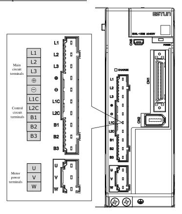
Take for example a product with a power rating of  $1kW\sim1.5kW$ . Products with power rating from 1.5kW to 3kW are similar in appearance and have the same components
