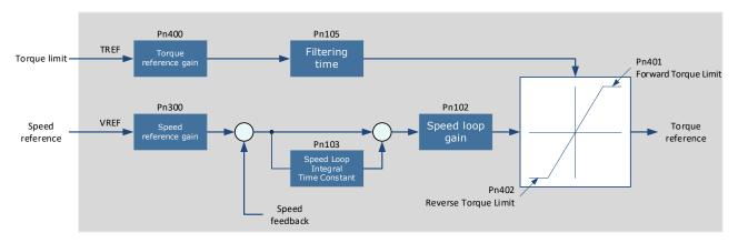
[Note] There is no issue with input voltage polarity of the analog voltage reference for torque limiting. The absolute values of both + and - voltages are input, and a torque limit value corresponding to that absolute value is applied in the forward or reverse direction.
