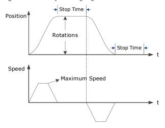
The Drive will operator the Motor repeatedly according to the parameter settings of the two operation patterns until the tuning is completed. You can set the parameters Pn164 and Pn168 to a negative value for reversing the Motor, so that there are four ways of the operation in the program jogging, as is shown in Figure 8-9.
