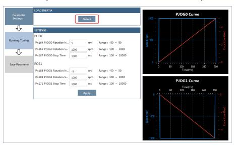
Step 5 Set the relevant parameters for the operation patterns POS0 and POS1.
