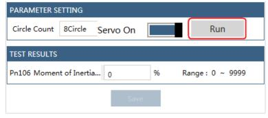
Step 6 When the **Load Inertia Identification** function has been completed, the result will be displayed in the textbox.
