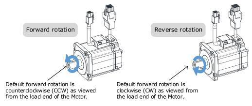
**NOTE**: The rotation direction of the Motor depends on the setting of Pn001.0 (CCW, CW). The figure above shows the default setting.
